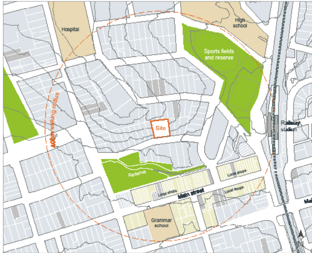
Figure 2-18 The neighbourhood scale outlines the urban grid and block structure including streets and open spaces, significant topography, heritage and civic and community uses. Proposals for individual or small groups of low rise medium density development sites should address this scale.
