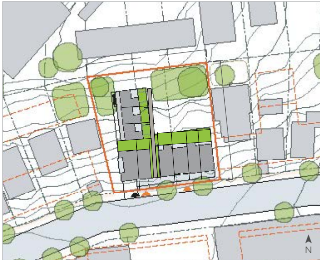
Figure 2-20 The site scale is a detailed analysis of the development's immediate context and should include the site itself, the street it addresses and surrounding properties. All proposals should address this scale.
