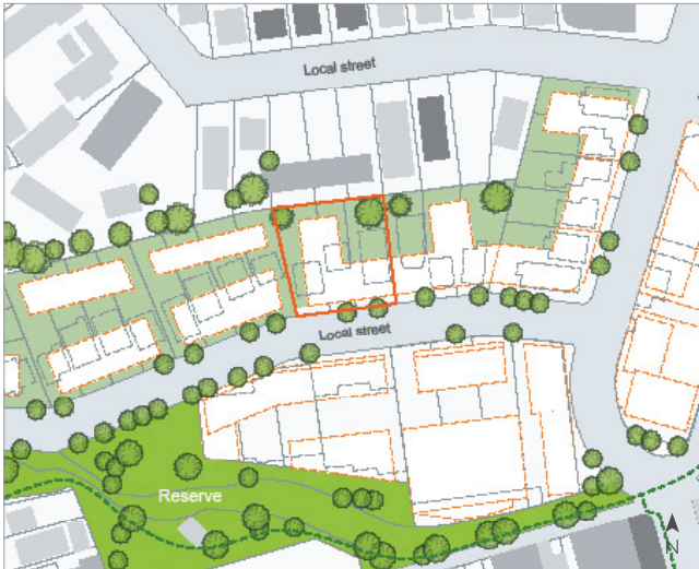
Figure 2-19 The streetscape scale helps understand the impact of proposed development on streetscape quality and should show heights, setbacks, driveways and existing street trees. All proposals should address this scale.
